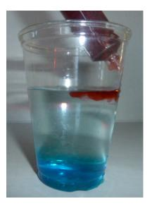
4. Fill a Styrofoam cup one half full with red hot water. Measure out 20 ml of hot water in the syringe. Hold the syringe against the side of the cup, but above the water, and drip the water down the side of the plastic cup. Again, this needs to be done very slowly to prevent mixing. Students should see that the hot water layered on top of the room temperature water because it is less dense.
